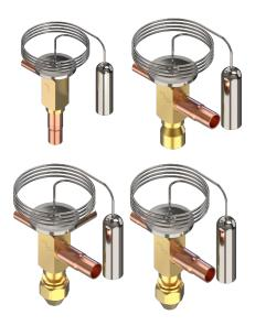
TD 1 / TDE 1 is a thermostatic expansion valve designed to regulate refrigerant injection into evaporators. The injection depends on the refrigerant superheat at the evaporator outlet, where the bulb must be placed.
