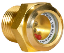
Figure 5: Sight glasses help determine quality of refrigerant and often include a moisture indicator. Ball valves are used to isolate refrigerant before servicing.
